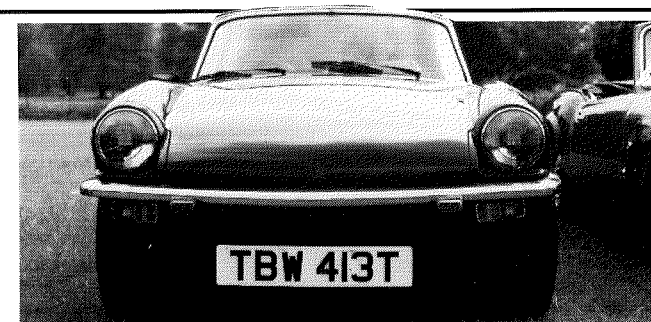
Fig.11. The number plate lowered below the radiator grille in a similar position to the Spitfire IV.
