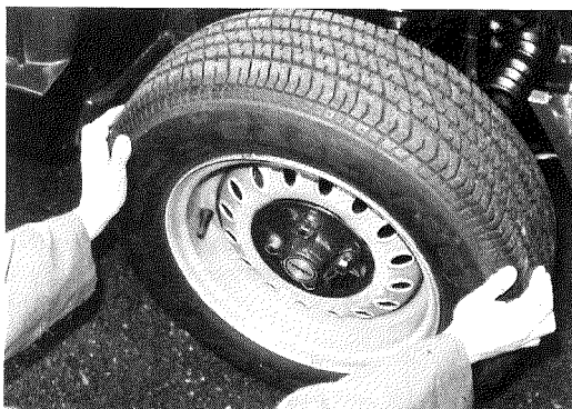
Fig.6. Wiggle wheel in and out to check for wear in track rod ends and steering rack
