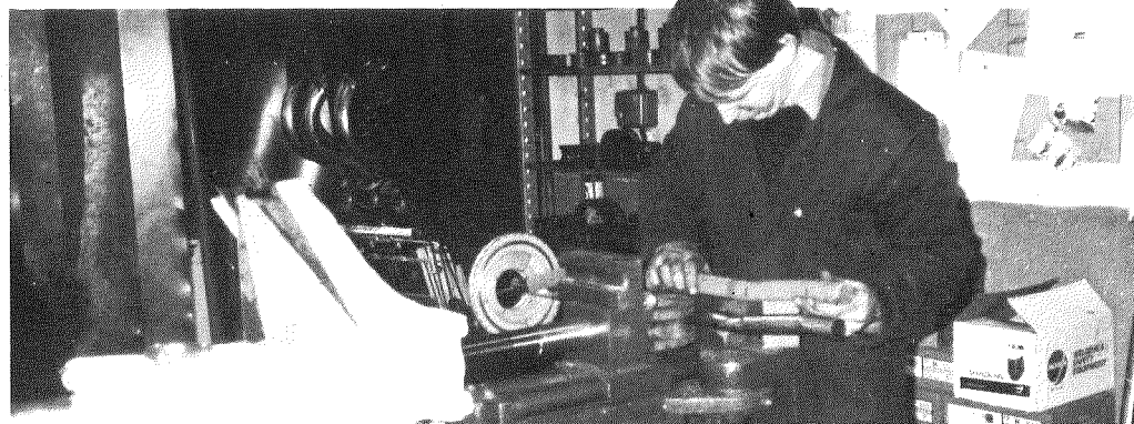
Fig.6. Pipe is 'Crush Bent' to original angles which work in degrees of bend and degrees of rotation.
