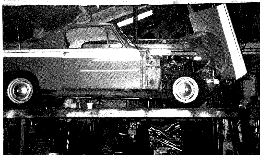
Fig.1. Car placed on lift, original system removed after noting fit, clearances and fitting kit.
