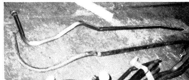
Fig.9. Completed downpipe (top) Mild steel (original) pattern below. Here you can see why the operators skill in interpreting angles is vital. As George said, having an actual vehicle to work to, means you can achieve a much more tailored fit. George 'improved' the angle around the gearbox filler to allow better access.
