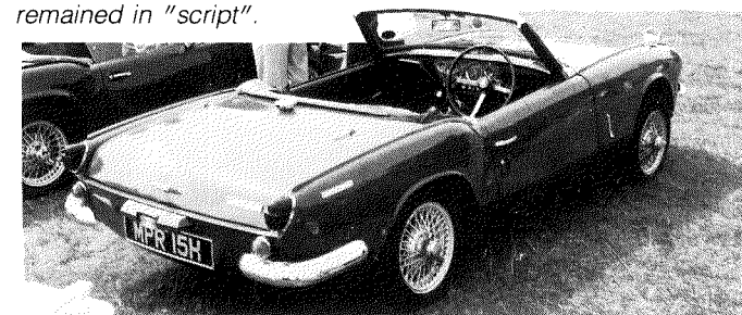
"Optional extra" wire wheels not only enhanced the car, but their greater 4½J width improved roadholding over the standard 3½J steels, especially when fitted with optional radial tyres.
