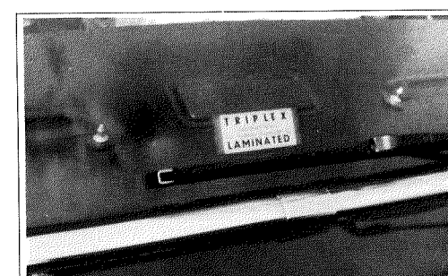
Fig. 18. Laminated windscreens were an option on early Spitfires becoming a standard fit on later cars.
