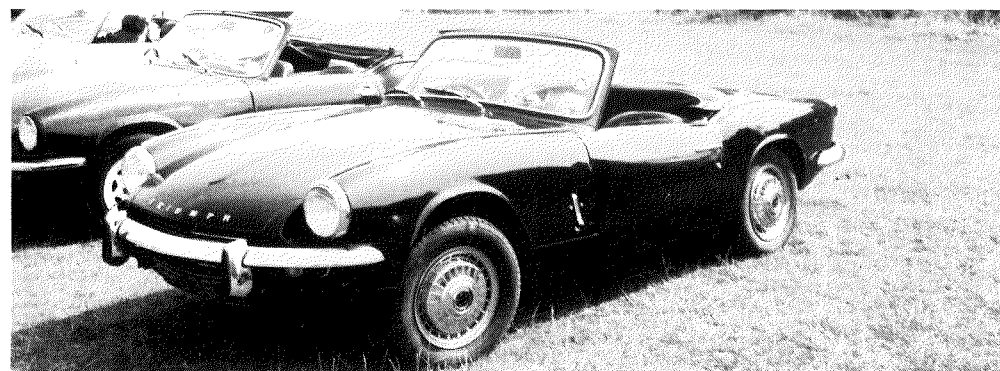
Top speed is reduced by around 5mph with the roof down. Most Mk3's use "turn catches" to secure the hood to the screen frame, though a small proportion are fitted with overcentre (Herald type) fasteners. Screen frames, originally in body colour, became matt black after October 1969. (The wheel trims shown here are non-standard).
