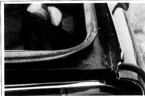
Fig.20. Early Spitfires were fitted with a boot seal that had to be stuck on. It was very flimsy, easily deforming and becoming unstuck.
