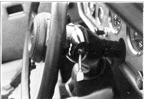
Fig.7. - FH 75,001 - FH 100,020 The early style steering column switchgear.
