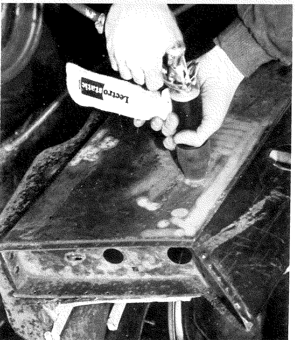
Fig. 6 A suitable test for the gun proved to be the new wing currently being fitted to my Vitesse which had a fair amount of surface rust. The nozzle should be pushed squarely and firmly against the work before pulling the trigger. As the name implies, the spot blaster is designed to clean away rust and old paint from small penny sized areas, a two to three second burst usually being sufficient to complete the job. However, with patience, larger envelope size areas can be cleaned back. It's very easy to start dragging the nozzle along the work surface but this leads to some wastage of abrasive so in practice it's best to blast a
