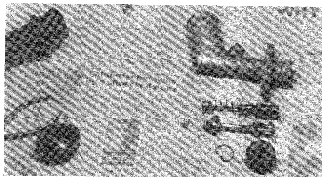
Fig.4 The constituent bits: cylinder body; inner piston assembly; push rod; circlip and dust cap. The bore should be cleaned using fresh brake fluid after which, inspect the surface walls and if there's evidence of any marks in excess of the general slight discoloration produced by the piston seal, it's probably best to replace the whole unit with new. If in any doubt replace the cylinder though usually it'll be OK.
